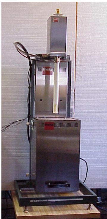
Measuring Stand in loading Position
